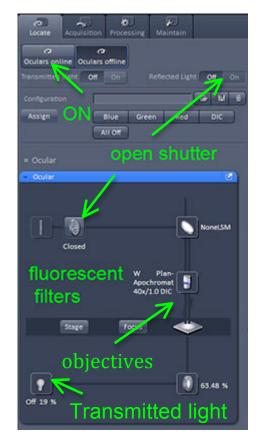
Alternatively, using the touchscreen, on the right column under the Home menu, you can turn on/off the RL (reflector light) Illumination and the TL (transmitted light) Illumination
