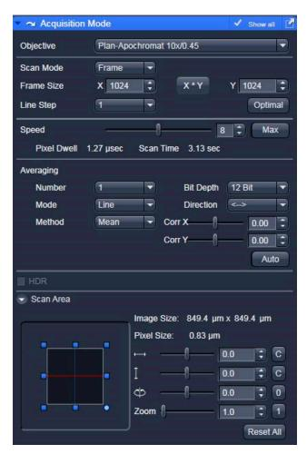
Averaging also improves the quality of the image because the repeated acquisition (line mode or frame mode) averages out the random noise. However, this is not an option for fast live imaging, e.g. with calcium green.
