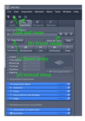
Set up the configuration in 4 ways: (a) load a \*.czi file and reuse its configuration, (b) choose from a preset configuration, (c) use "Smart Setup", or (d Set up the configuration in 4 ways: (a) load a \*.czi file and reuse its configuration, (b) choose from a preset configuration, (c) use "Smart Setup", or (d) manual setup.
